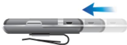
2. Place the Speakerphone with sun-visor mount onto the sun visor of your car.
