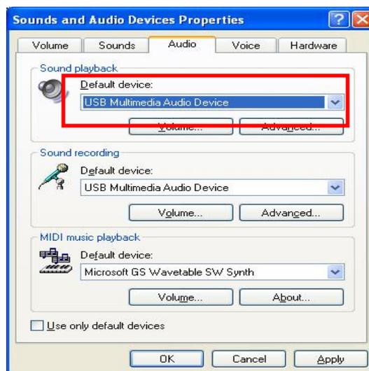
For Vista users, right click on the Speaker icon at the bottom right corner of your system tray, then make sure the “**2- USB Multimedia Audio Device**” is checked then click **Set as Default Device** and **OK**.
