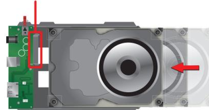
3. Align the hard drive relative to the screw holes of the board
