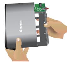
2. Once you have removed the board from the inside of the enclosure, slide your hard disk into the connector attached to the board as shown below:
