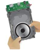
4. After the drive has been connected to the board, use the HDD screws (CM#6 x 6 provided) to fasten the drive to the base and to ensure the drive is locked in securely.
