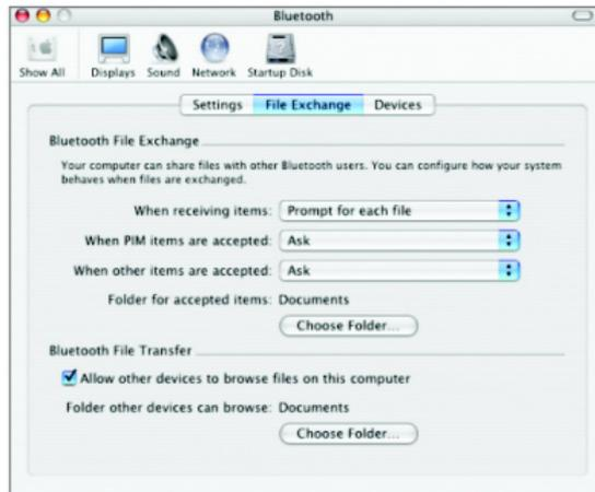
5. On the devices tab, you may pair with your Bluetooth device(s) or search for other Bluetooth devices available to you. In this example, we will connect to a Bluetooth cell phone. The procedure for other Bluetooth devices is similar. Simply follow the Bluetooth setup assistant.
