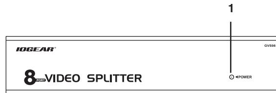
1. Power LED light to indicate the unit is receiving power.
