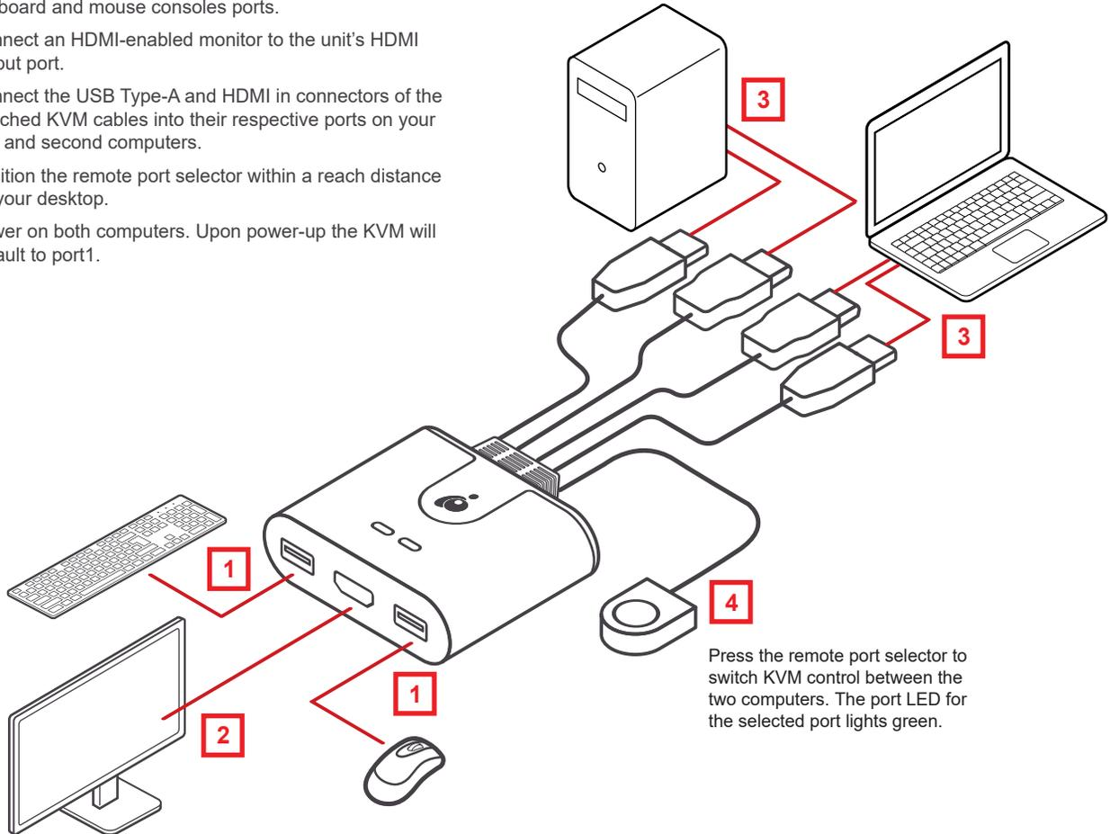
Press the remote port selector to switch KVM control between the two computers. The port LED for the selected port lights green.
