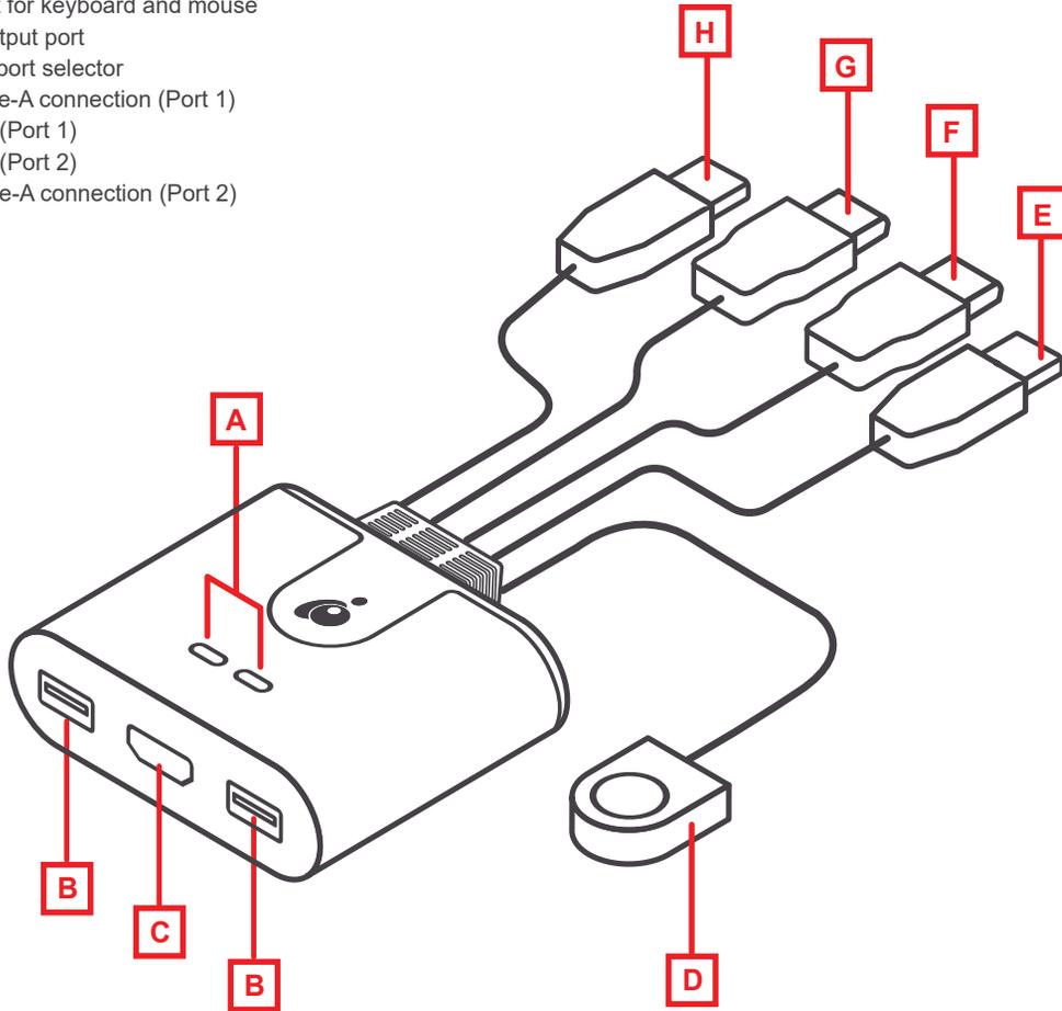
1. Connect your keyboard and mouse to the unit's USB keyboard and mouse consoles ports.
