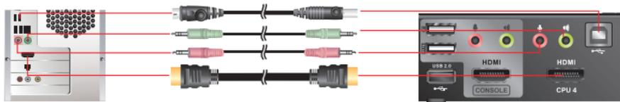
\*If your source device has a DVI output instead of HDMI, please connect the HDMI (F) to DVI (M) Adapter (Model No: GHDMIFDVM) between your source device and your HDMI cable.
