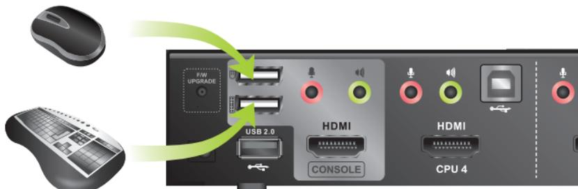
\*If you are using PS/2 keyboard and mouse, please use the included PS/2 to USB converter. Simply connect the PS/2 keyboard and mouse to the PS/2 keyboard and mouse port from the converter, then connect the USB port to the console USB keyboard port.
