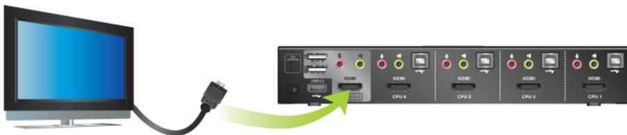
\*If your display has a DVI input instead of HDMI, please connect the HDMI (F) to DVI (M) Adapter (Model No: GHDMIFDVIM) between your HDMI cable and your DVI connection from your display.
