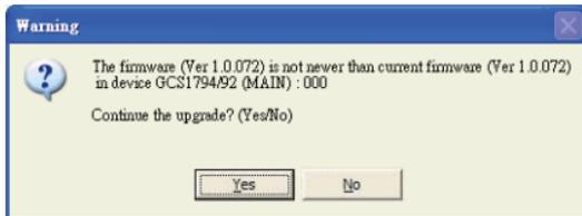
Note: If you did not check the “Check Firmware Version” checkbox, utility will perform the upgrade automatically no matter what version of firmware you have in the KVM.
