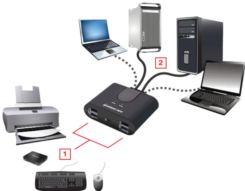
Note: The GUS402/GUS404 are hot-swappable and do not require the computers to be turned off during connection, or when attaching devices to the USB ports.
