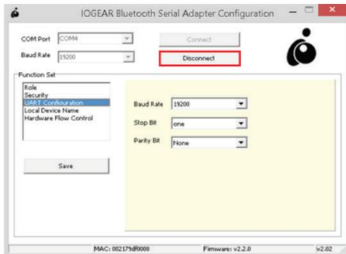
18. Push the CFG / RST button for one second and release. The orange Mode LED light will turn off. You have successfully completed configuration of the Bluetooth Serial Adapter.
