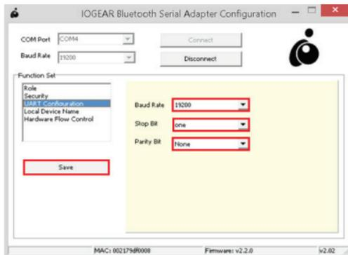
17. Click on the **Disconnect** button and close the IOGEAR Bluetooth Serial Adapter Configuration tool.
