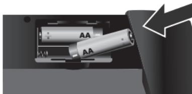
\*Note: Please make sure the batteries are installed properly as the directions that are indicated inside the battery tray
