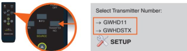
2. Select **SETUP** menu by using the **Up / Down** buttons; press **OK** to select.
