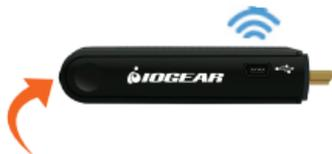
2. The transmitter is in Pairing Mode once the Power LED flashes slowly (1 flash/sec).
