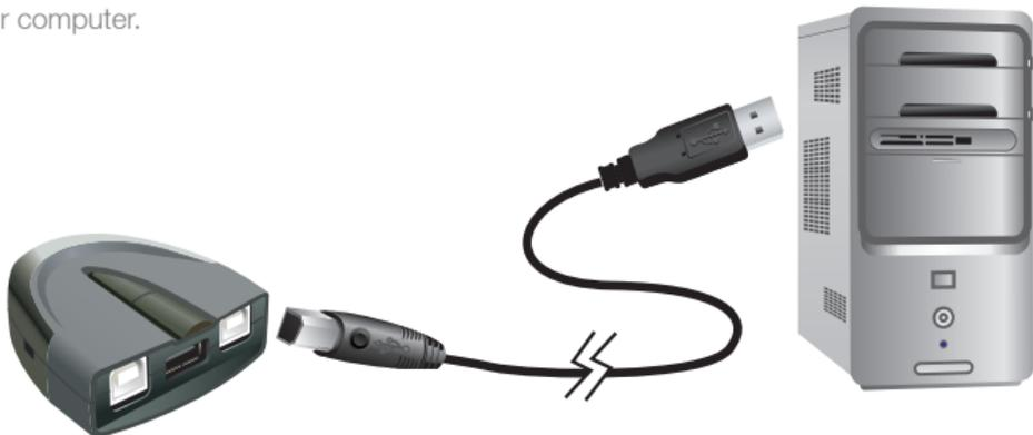
3. Connect the USB Type A connector of the USB cable from your USB device to the Type A port on the GUB231 or GUB431.
